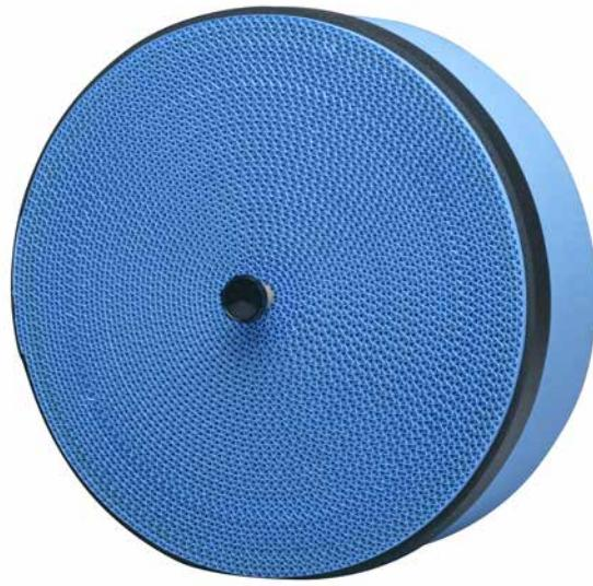
Donaldson PowerCore Spider-Web filter media uses a proprietary blend of cellulose and fully synthetic man-made fibers to create a multi-layer moisture and humidity resistant premium filter media substrate. A surface coating of Donaldson Spider-Web fine fibers is added for high efficiency against small particles. By controlling the material, shape and diameter of the fibers, this multi-layered media is designed to perform effectively in most environments.
