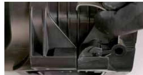
Unlock the pre-cleaner cover by pressing the side clips. Open the pre-cleaner cover to clean the chamber.
