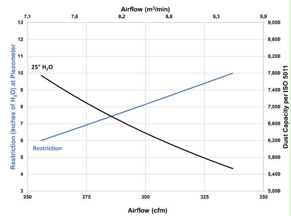
\*Results generated using laboratory testing pursuant to ISO5011. Actual performance during use may vary depending on multiple factors, including specific product configuration, external conditions and application.
