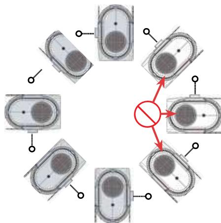
**Non-Scavenged System Mounting with Vacuator™ Valve** (shaded air cleaners indicate proper mounting positions)
